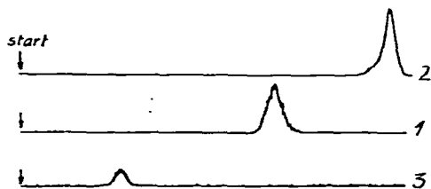
Fig. 1. Separation of uracil (1), dihydrouracil (2) and \beta -ureidopropionic acid (3) by TLC with Kieselgel D plates in the solvent system chloroform-methanol-acetic acid (100:5:1) at 4° (continuous sandwich conditions, 12 h).
